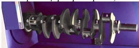
Fig. 1. 1, 2, 3, 4, 5, 6 – fusuri paliere, a, b, c, d, e – fusuri manetoane
