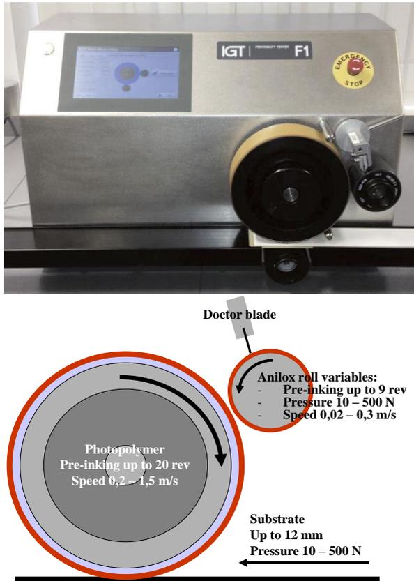
**Fig. 1. IGT F1 Printability Tester Operation.**
