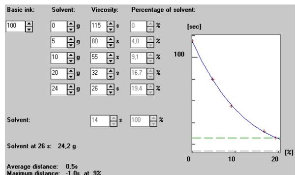
**Fig. 2. Viscosity calibration curve for a 26 s flow time.**
