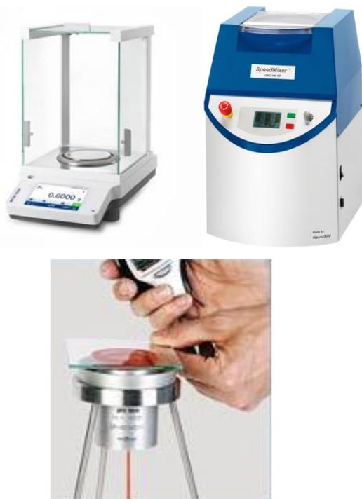
**Fig. 3. Operation of analytical balance, ink speed mixer and flow cup.**
