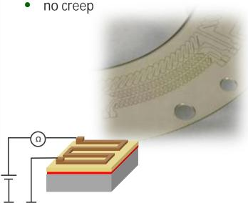
Innovation: Sensotect® coating for measurement of surface deformations inside transmission
