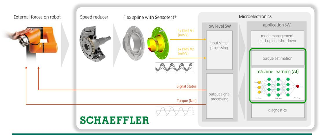
Innovation: fully integrated torque measurement based on Sensotect & embedded AI (machine learning)
